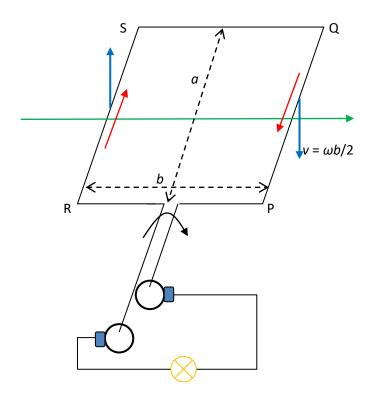
Think of the "rod" PQ that moves with speed v cutting magnetic field lines. We know that in this case there is a motional emf *BvL*. Thus the induced emf across PQ is  $\mathcal{E}_{PQ} = Bva = B\frac{\omega b}{2}a = \frac{B\omega A}{2}$ . End P is positive and end Q is negative. This means the induced current is from Q to P (right red arrow).
