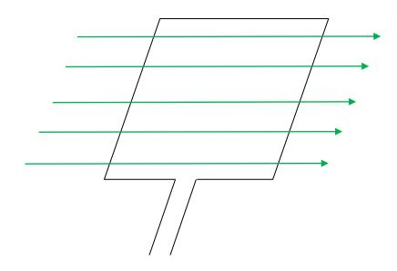
In general, the flux will be given by  $\Phi = BA\cos(\omega t)$  and so the induced emf in the loop will be  $\varepsilon = -\frac{d\Phi}{dt} = BA\omega\sin(\omega t)$ . The maximum induced emf is thus  $\varepsilon_{max} = BA\omega$ . How can we get this result without calculus?
